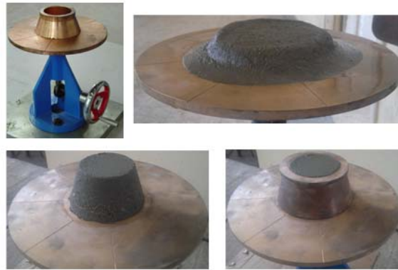
Figure (2): Flow table for mortar workability
