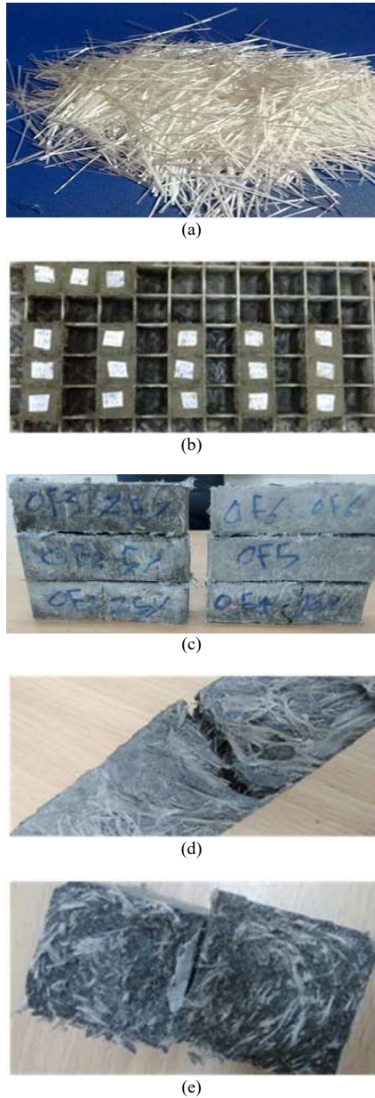
Figs. 1. Elements and samples used in compression and bending strength experimentations. (a) Alkali-resistance glass fibers of filament thickness 14 to 20 \mu\text{m} , (b) Molds made of a non-absorbable material with 50.5×50.5×50.5 mm, (c) Remolded f_{bf} beams before curing (d) Cracked f_{bf} beams after bending experimentation, and (e) f_{bf} cube specimens after 24 hours of casting
